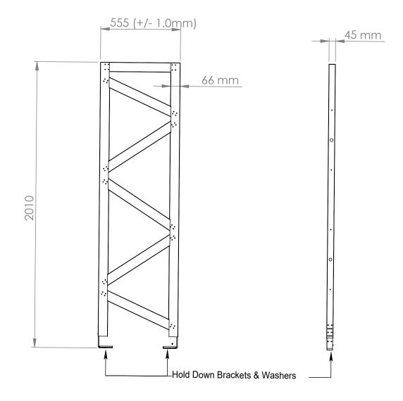
Detailed in the drawing below is the GBF600S as it must be constructed within the timber framing to provide the described wind and earthquake performance values.
